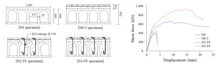
Fig. 1 Comparison of shear behavior of HCSs with and without strengthening
